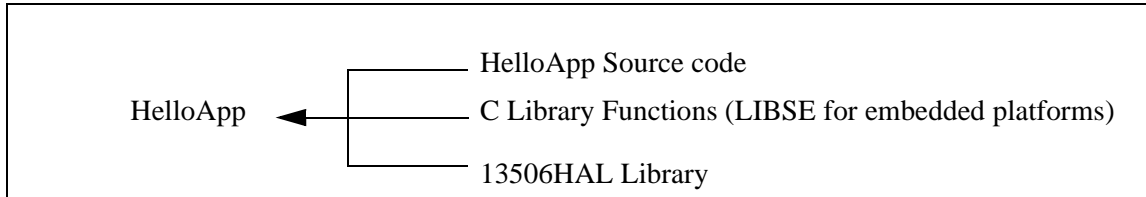
Figure 14-1: Components needed to build 13506 HAL application
